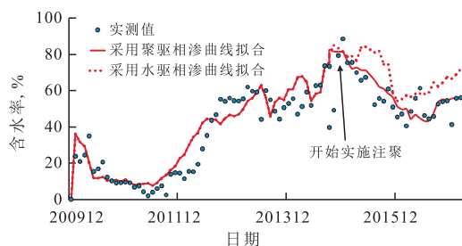
图5 注聚试验区不同相渗曲线含水率拟合情况对比 Fig. 5 Comparison of water content fitting of different phase permeability curves in polymer injection test area
