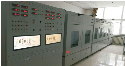
图1 非常规储层动态模拟系统装置 Fig. 1 Dynamic simulation experiment system of unconventional reservoir
