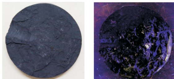
图1 层理缝含油显示(HA14井,2 219.95 m,黑色泥岩) Fig. 1 Layer fracture with oil display (well HA14, 2 219.95 m, Black mudstone)
